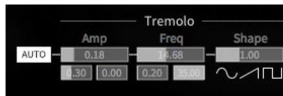
**Amp:** The Amplitude controls the intensity that the Tremolo effect has on the general sound. The Amp control has a **Minimum** and **Maximum** control underneath its slider which delimits the range of intensity. *Note: This function is exclusively working when AUTO Mode is turned on.*
