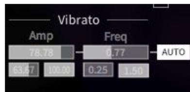
**Amp:** The Amplitude controls the intensity of the Vibrato effect on the general sound. The Amp Control has a **Minimum** and **Maximum** control underneath its slider which delimit the range of the Amplitude. *Note: This function is exclusively working when AUTO Mode is turned on.*
